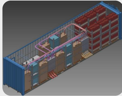
Containerized Battery Bank with Hybrid Solar Inverter
